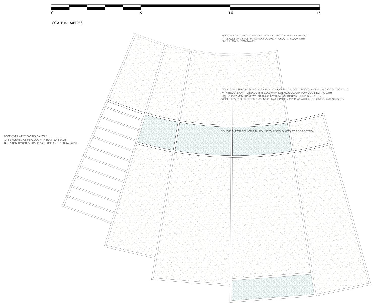
DOUBLE GLAZED STRUCTURAL INSULATED GLASS PANELS TO ROOF SECTION
